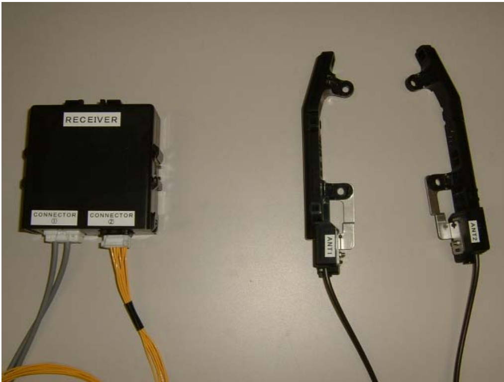
Receiver and two antennas
