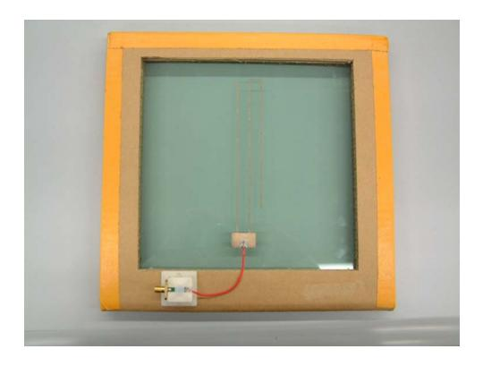
The antenna is installed in vehicle's rear glass. This ANT pattern is similar to actual ANT pattern.
