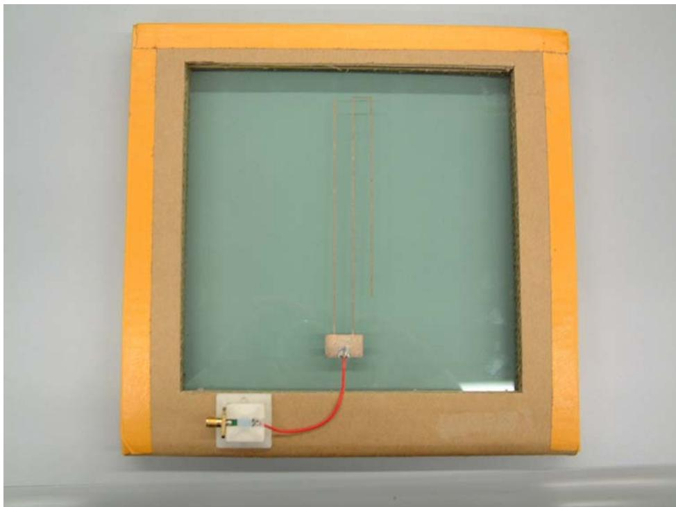
The antenna is installed in vehicle's rear glass.
