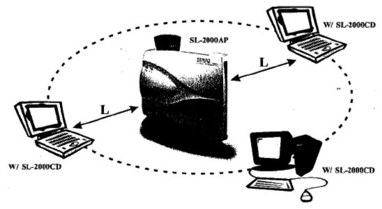
Figure 1-3 Extended-range independent WLAN using AP as repeater
