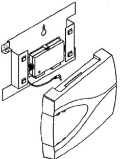
Figure 2-6 Attaching the AP
