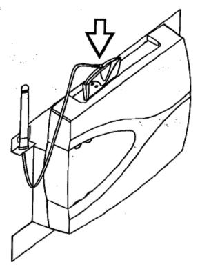
Figure 2-9 Connect the external antenna
