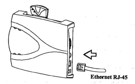
Figure 2-8 Connecting the Ethernet cable
