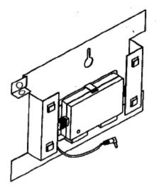
Figure 2-5 Mounting the power adapter
