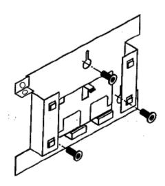
Figure 2-4 Mounting the bracket
