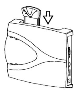
Figure 2-7 Inserting the PC Card
