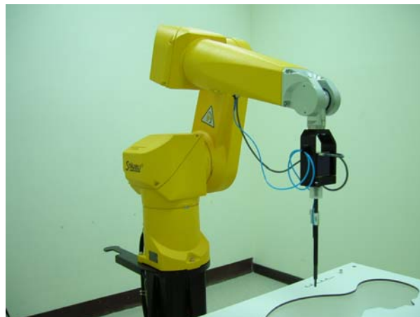
Fig. 5.2 Probe setup on robot
