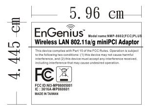
P/N:6710A0343010 LABEL FREQUENCY 59.6x44.45mm EMP-8602 (FCC) PLUS LFP
