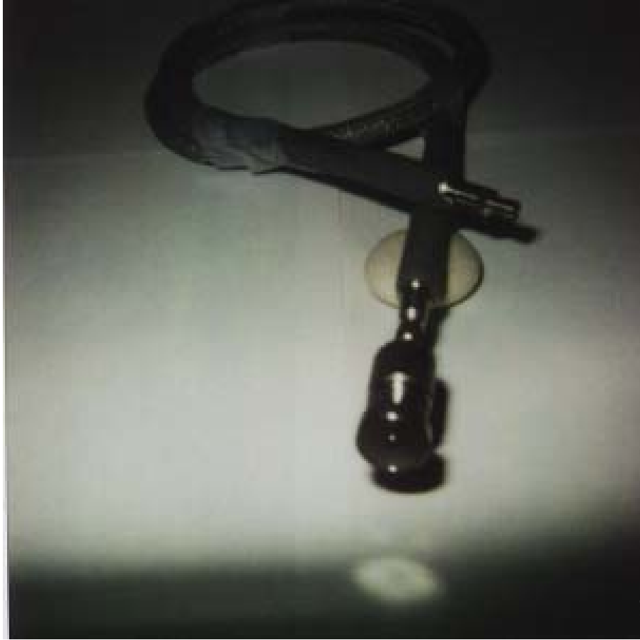
Fig. 11. Photograph of the Hewlett Packard Model 85070B Dielectric Probe. This is an open-circuited coaxial line probe.
