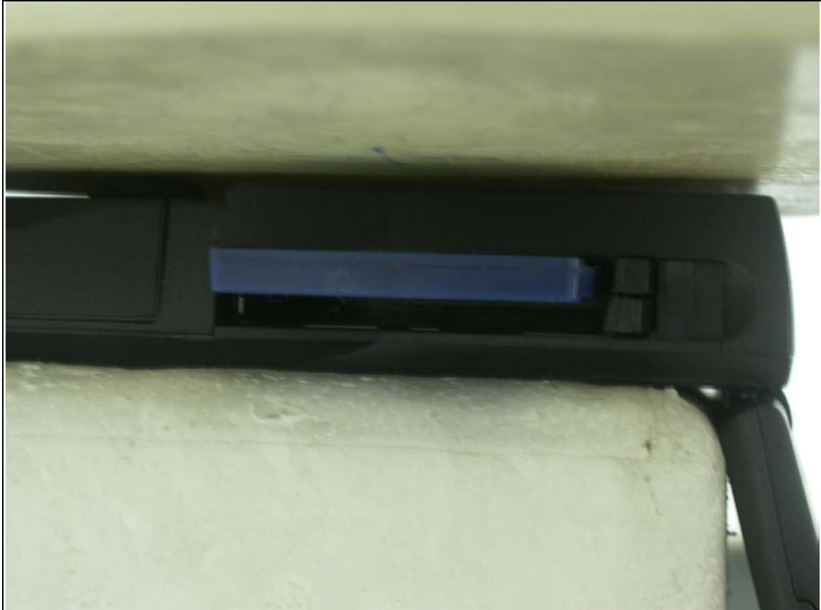
Bottom of the EUT to the flat phantom distance 13mm
