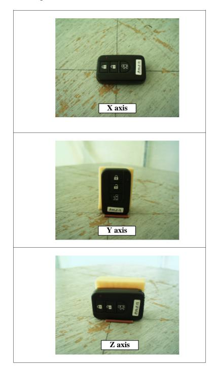
Worse case X axis (30MHz – 4.5GHz, Measurement antenna Polarization: Horizontal) Worse case Y axis (30MHz – 4.5GHz, Measurement antenna Polarization: Vertical)
