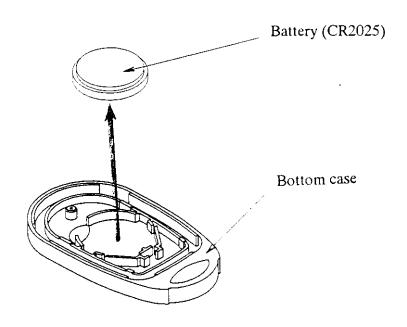
When the Remote Keyless Entry Transmitter's Battery begins to get weak, replace the Battery as soon as possible.
