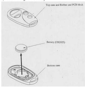
To replace When the Remote Keyless Entry Transmitter's Battery begins to get weak, replace the Battery as soon as possible.
