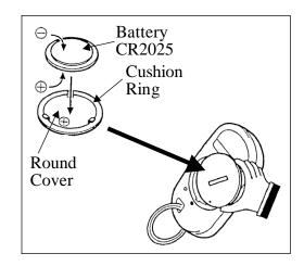
Remove the old Battery and note the polarity. Make sure the polarity of the new Battery is the same (+ side facing up), then insert it in the Transmitter.
