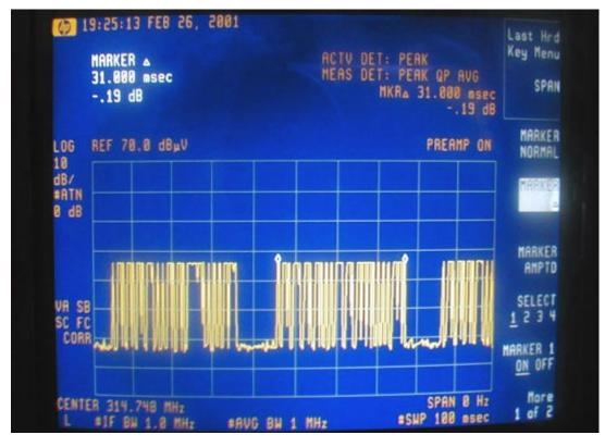
**Receiver: Picture of the Duty Cycle Test**
