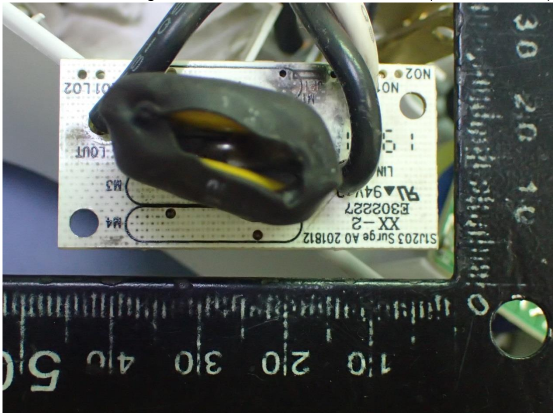
Figure 18 For Surge Protector 560J Model, Internal View (PCB Front View)
