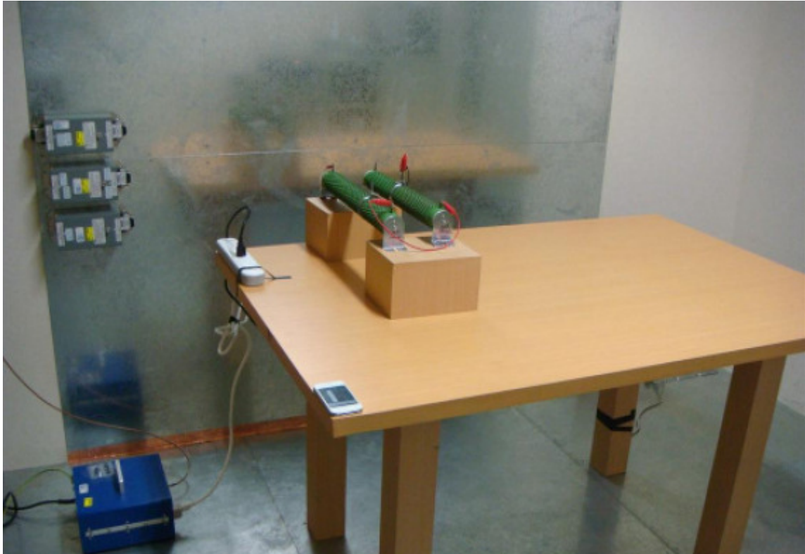
Photograph 5: Set-up for for Mains Conducted testing Back
