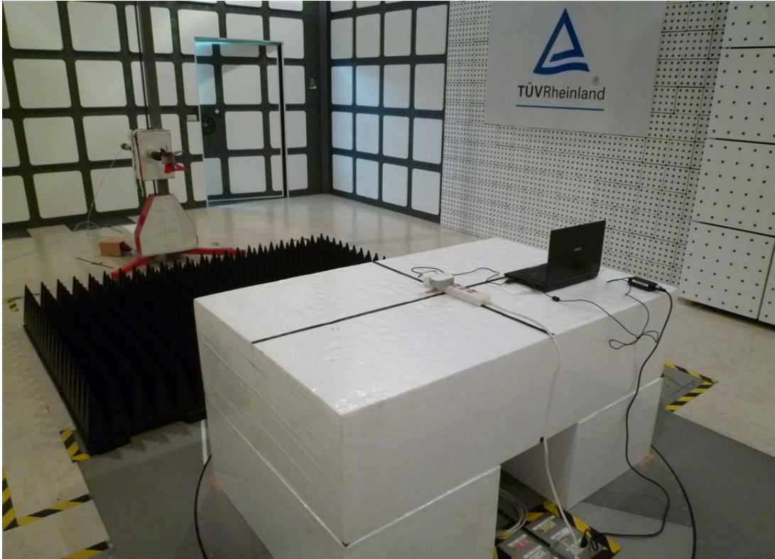
Photograph 4: Set-up for Conducted testing
