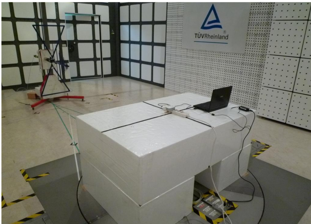
Photograph 2: Set-up for Spurious Emissions (Back View 1)
