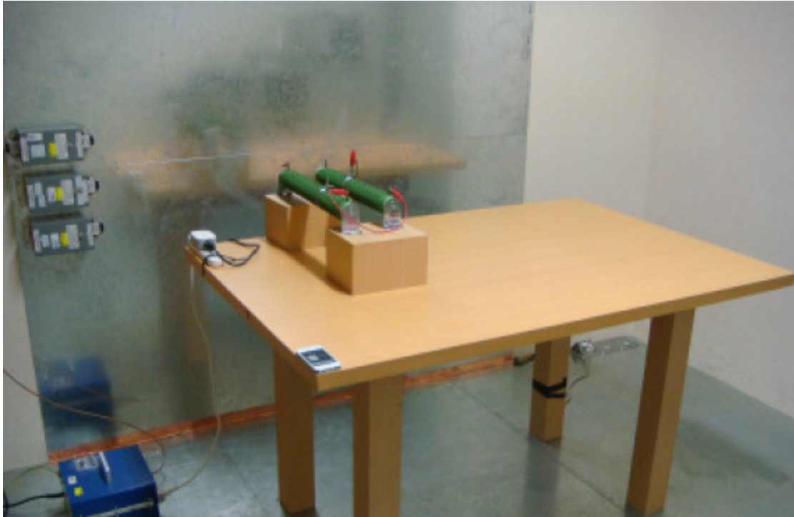
Photograph 5: Set-up for for Mains Conducted testing Back
