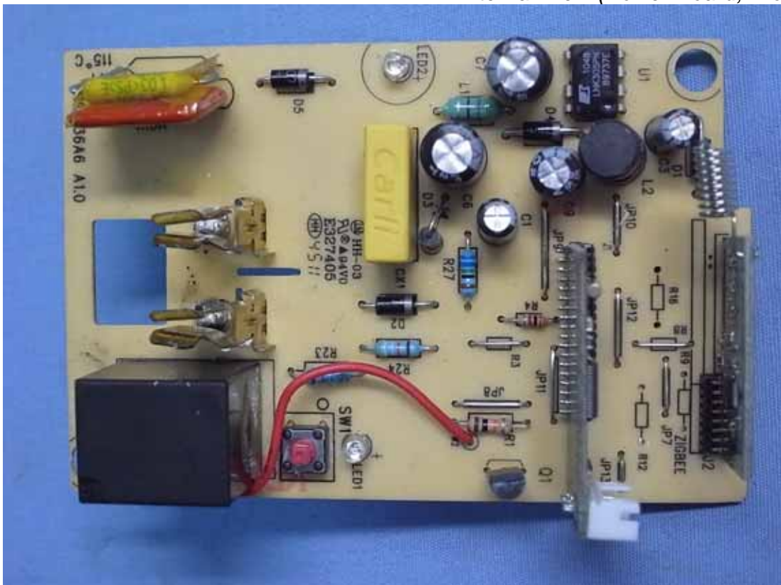
Photo 6 Internal View (Power Board, Front View)
