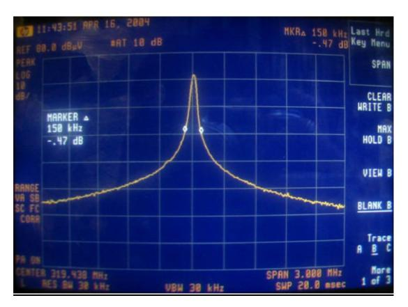
Plot of the Transmitter Bandwidth Measurement
