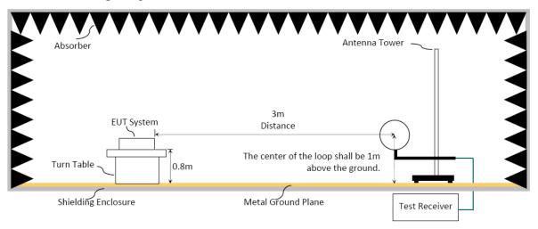
6.1.3. Setup Diagram for 30-1000MHz
