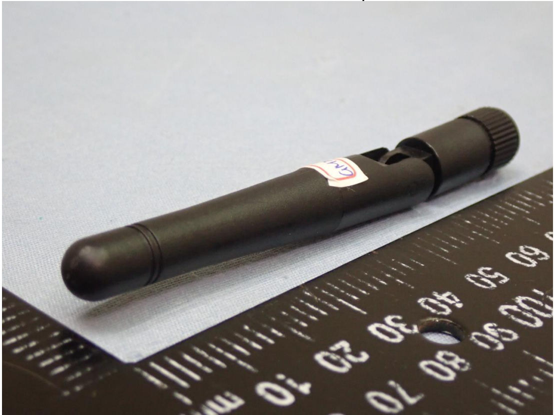
Figure 21 Dipole Antenna, Front View
