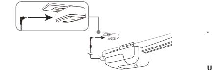
**3** Connect the power to your garage motor by plugging it back into the ceiling power outlet. If you turned the power to your garage off through the circuit
