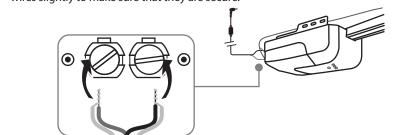
**D** Repeat steps B-C to connect the second motor control cable.
