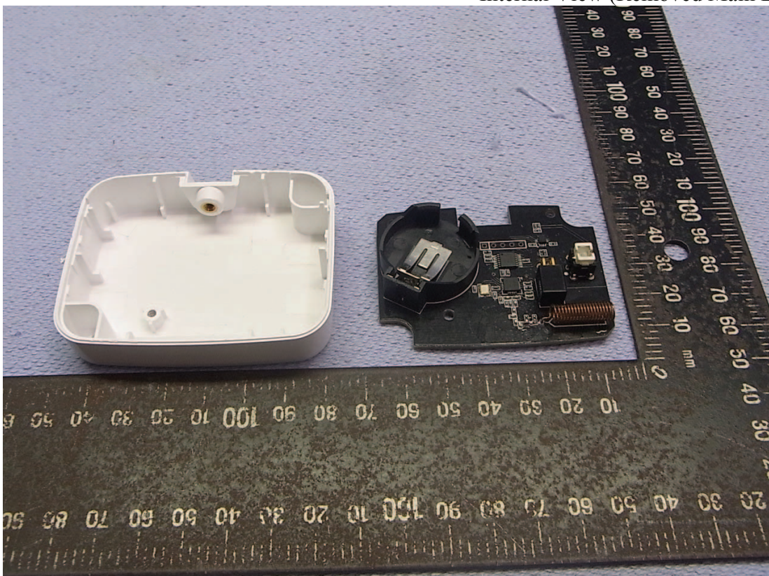
Figure 6 Internal View (Removed Main Board)
