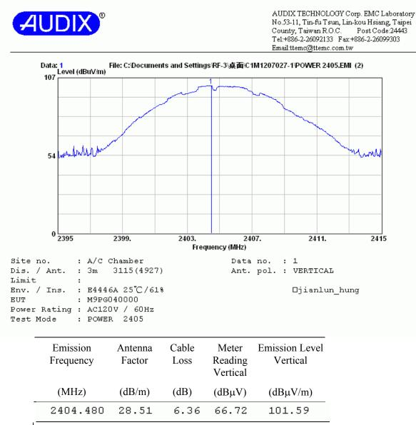
Remarks: 1. Emission level=Antenna Factor + Cable Loss + Reading.
