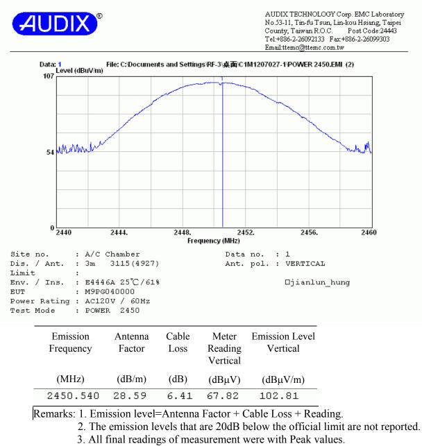
4. The pre-amplifier factor has been subtracted by test program actively.
