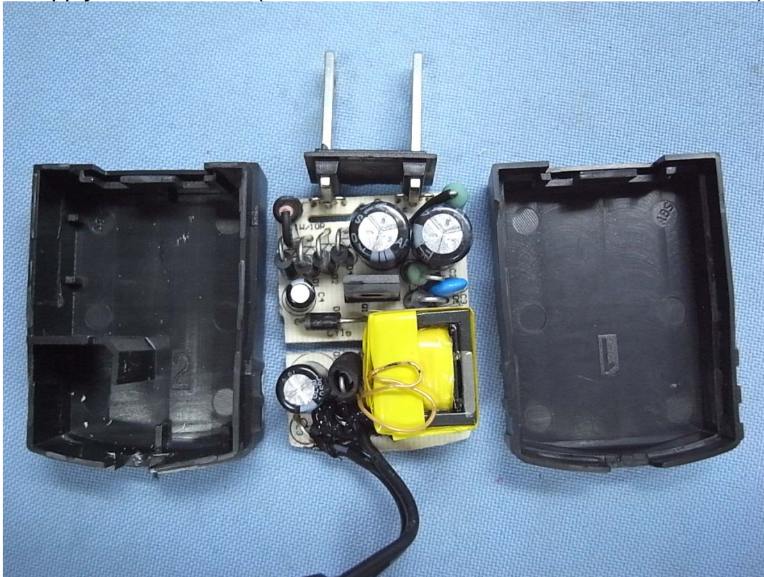
Figure 12 I.T.E Power Supply, Internal View (Removed Covers and Main Board, Front View)
