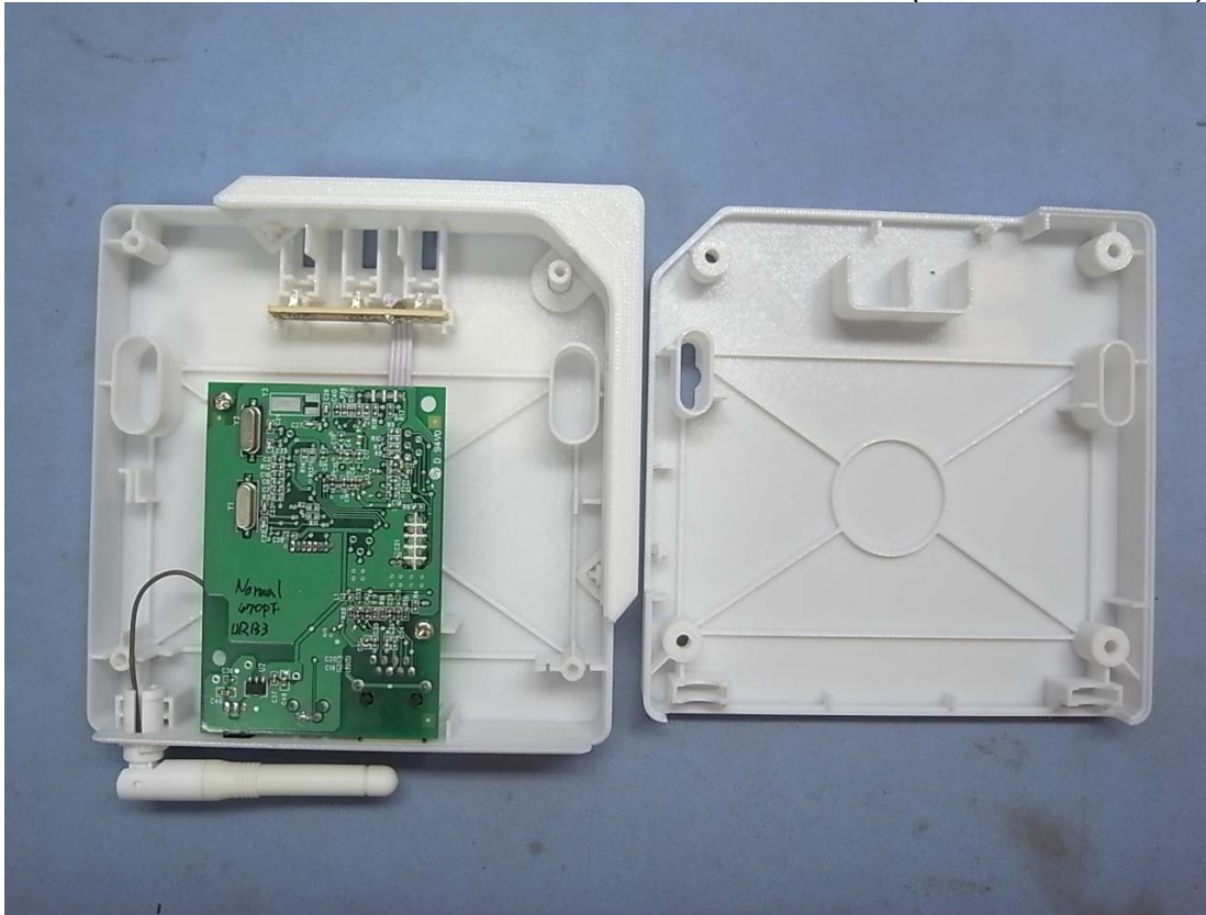
Figure 5 Internal View (Removed Cover)
