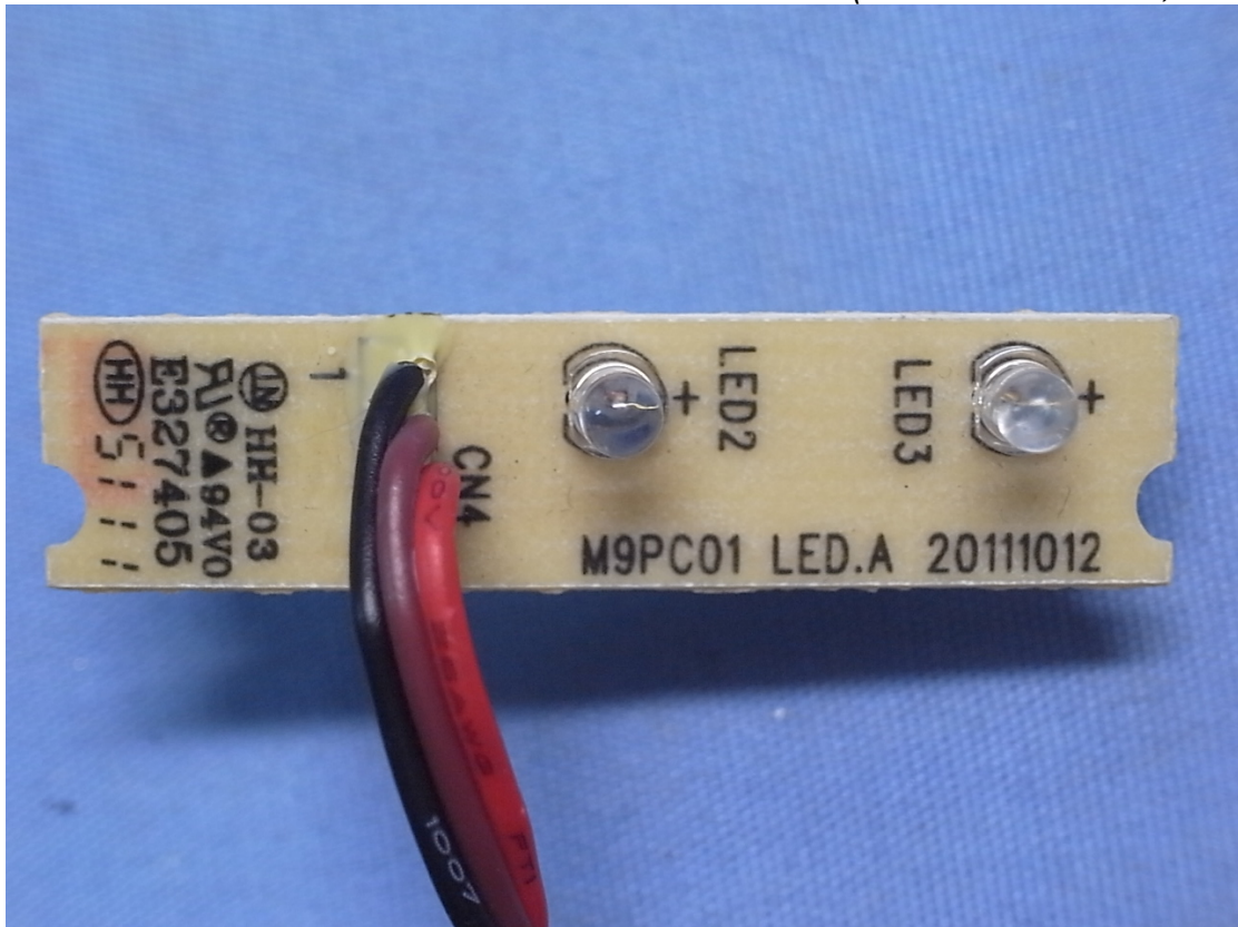
Photo 11 Internal View (LED Control Board, Front View)
