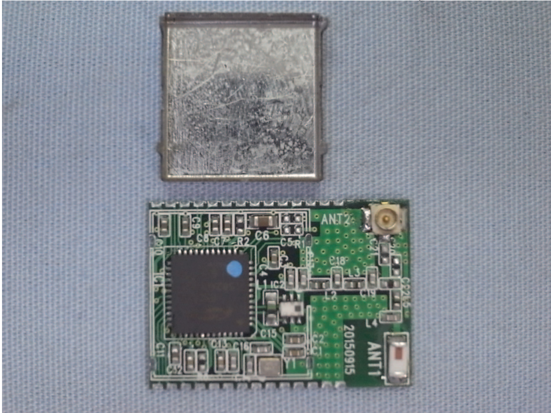
Figure 3 Internal View (Removed Shielded Cover)
