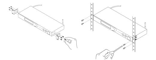
Step 1. Use included thumb screws to attach rack ears to power center.
