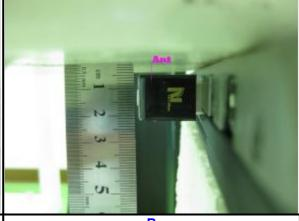
The bottom of the EUT faces to the phantom with 5mm-separation distance.
