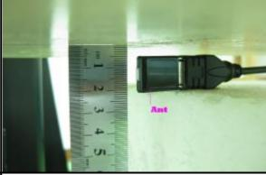
The front of the EUT faces to the phantom with 5mm-separation distance.
