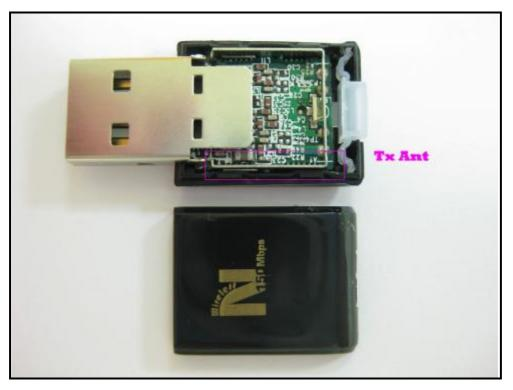
**NOTE:** TX diversity function is not supported for this product .Only one antenna can transmit.
