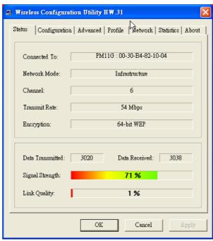
There are two dialog boxes showing the data transmitted and the data received. The two signal lines show the Signal Strength and the Link Quality of the device.
