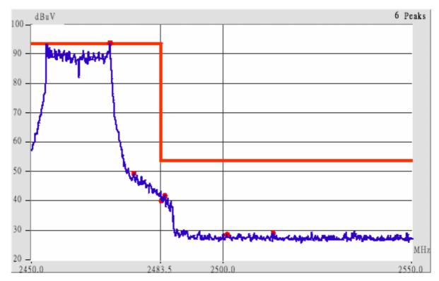
Undetachable antenna, 802.11g channel 11 (The Highest one in the frequency bands)
