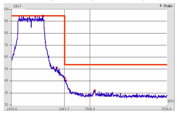
Detachable antenna, 802.11g channel 11 (The Highest one in the frequency bands)
