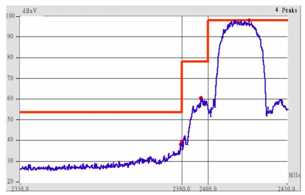
Undetachable antenna, 802.11b channel 1 (The lowest one in the frequency bands)
