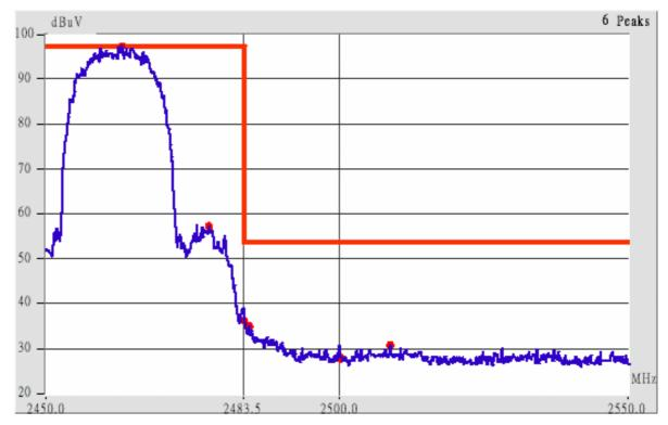
Undetachable antenna, 802.11b channel 11 (The Highest one in the frequency bands)
