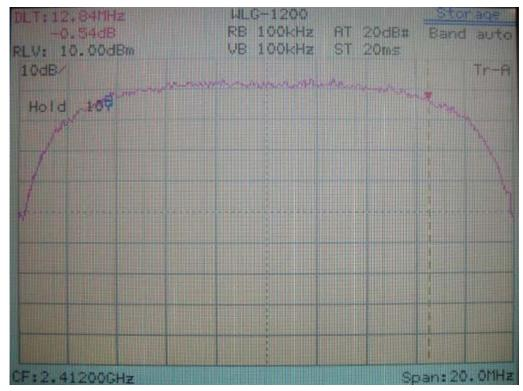
802.11b Channel 1: 12.84MHz (The minimum 6dB BW at least 500kHz)
