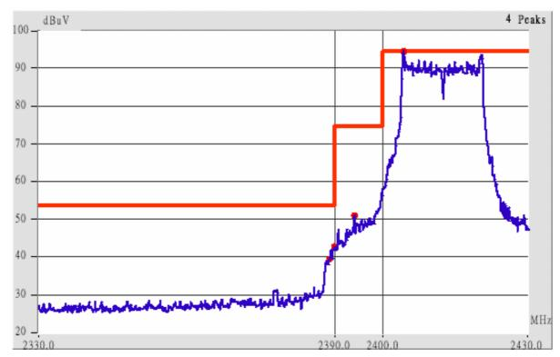
Undetachable antenna, 802.11g channel 1 (The lowest one in the frequency bands)
