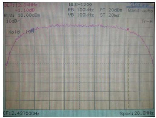
802.11b Channel 6: 12.84MHz (The minimum 6dB BW at least 500kHz)
