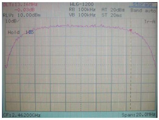
802.11b Channel 11: 13.16MHz (The minimum 6dB BW at least 500kHz)
