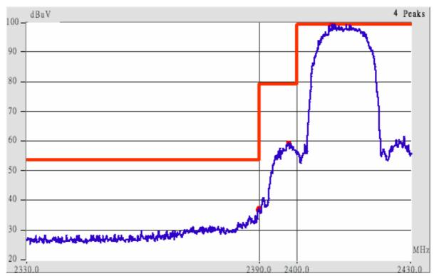
Detachable antenna, 802.11b channel 1 (The lowest one in the frequency bands)
