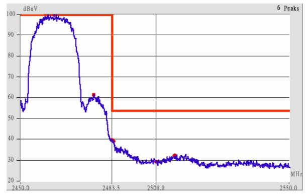
Detachable antenna, 802.11b channel 11 (The Highest one in the frequency bands)
