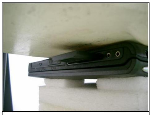
The bottom of the EUT face to the phantom with 10mm-separation distance.
