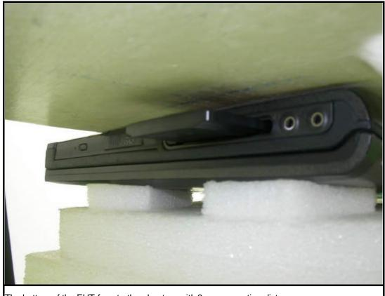
The bottom of the EUT face to the phantom with 8mm-separation distance.
