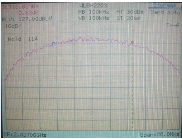
6dB Bandwidth of Channel 6: 8.88MHz (The minimum 6dB BW at least 500kHz)
