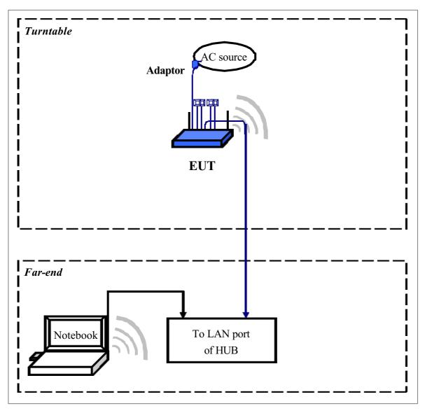
The tests below are carried with the EUT transmitter set at high power in TDD mode. The EUT is forced to select of output power level and channel number by computer.
