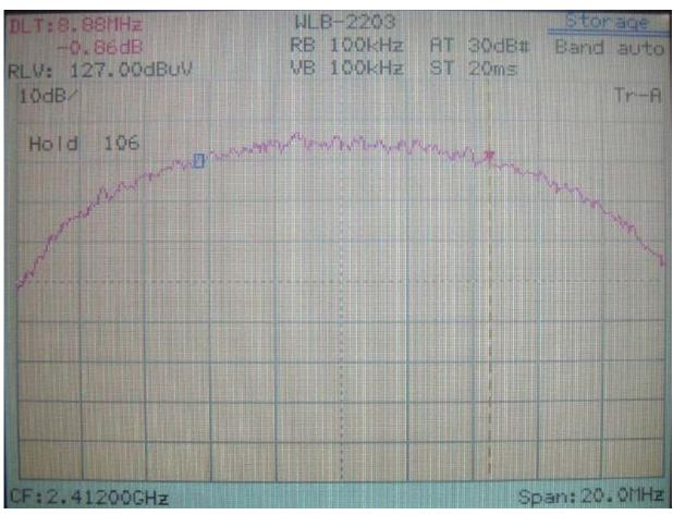
6dB Bandwidth of Channel 1: 8.88MHz (The minimum 6dB BW at least 500kHz)
