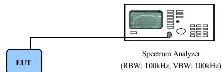
P.S.: The computer to control the EUT at maximal power output and channel Number and set antenna kit
