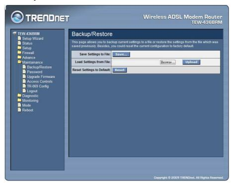
**Save Setting to File:** Click the "Save Setting to File" button to save current settings of the WLAN ADSL Router to local computer.
