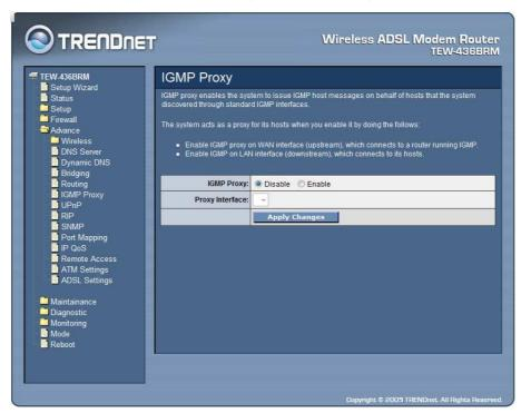
**IGMP Proxy:** Select to enable or disable the IGMP proxy feature on the WLAN ADSL Router.
