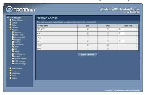
**LAN:** Checked the services on the LAN column to allows the services access from LAN side.
