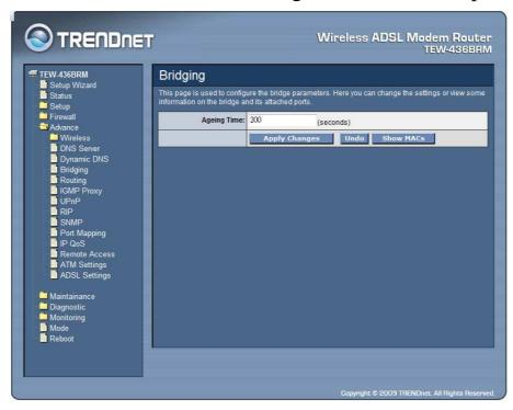
**Aging Time:** Set the Ethernet address ageing time, in seconds. After [Ageing Time] seconds of not having seen a frame coming from a certain address, the bridge will time out (delete) that address from Forwarding DataBase (fdb).
