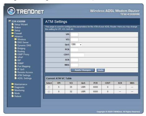
**VPI:** Virtual Path Identifier. This is read-only field and is selected on the Select column in the Current ATM VC Table.
