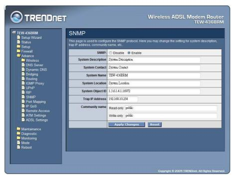
**SNMP:** Enable or Disable the SNMP feature on the WLAN ADSL Router.
