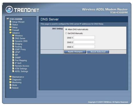
**Attain DNS Automatically:** Select this item if you want to use the DNS servers obtained by the WAN interface via the auto-configuration mechanism.
