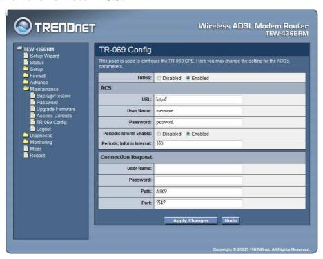
**TR069:** Enable or Disable the TR-069 feature on the WLAN ADSL Router.
