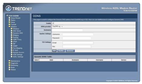
**Enable:** Checked to enable this registration account for the DNS server.
