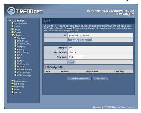
**RIP:** Select to enable or disable the RIP feature on the WLAN ADSL Router.
