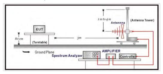
Above 1GHz Test Setup:
