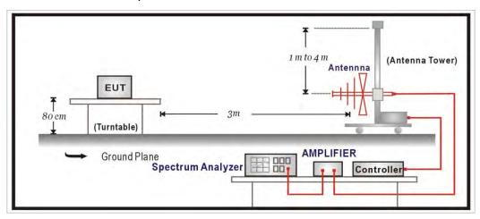
Above 1GHz Test Setup:
