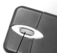
LED lights up: desktop mode LED goes out : in-air mode
