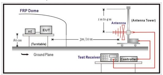
Above 1GHz Test Setup:
