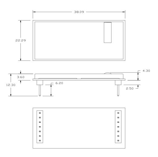
Unit: mm Tolerance: +/- 0.2 mm
