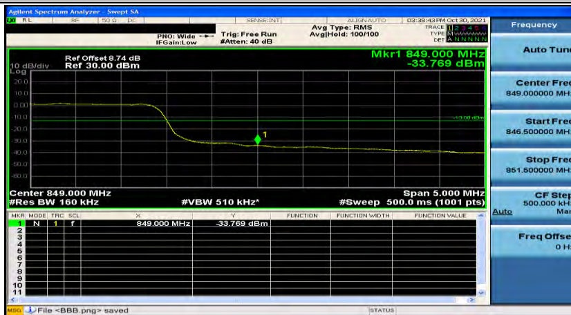
(Channel Bandwidth: 15 MHz)_HCH_ DFT-s Pi/2 BPSK _75RB#0
