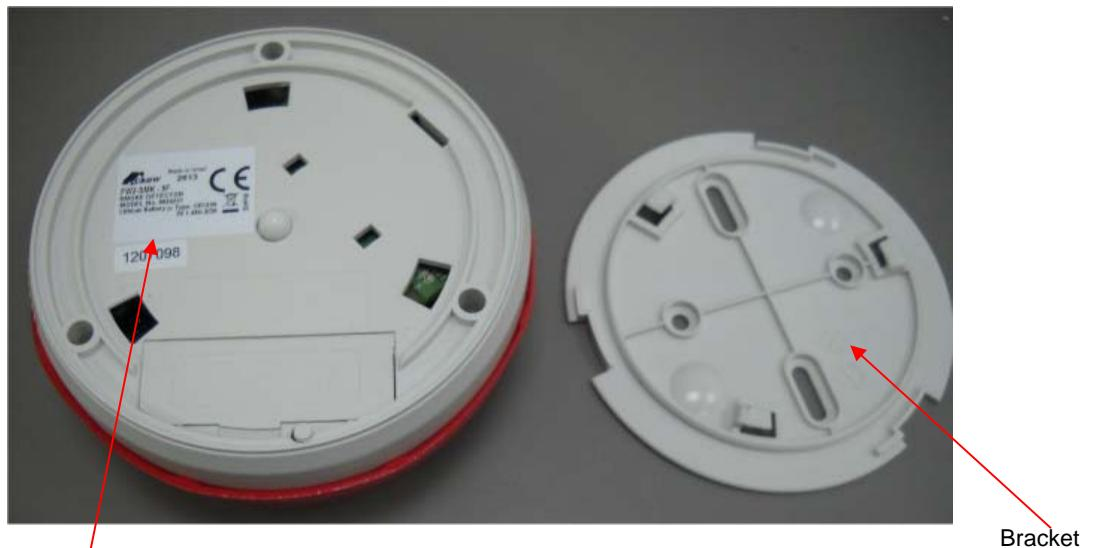
Label with **FCC ID:NFC-FW2SMK9F** is located at the rear side panel. The statement according to FCC part 15 §15.19(a)(3) is placed in Installation Instructions, page 4 (Application exhibit User\_manual\_25157).
