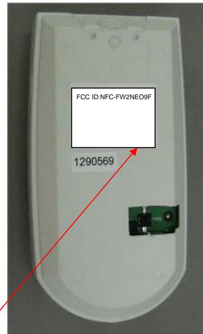
Label with **FCC ID:NFC-FW2NEO9F** is located at the rear side panel. The statement according to FCC part 15 §15.19(a)(3) is placed in Installation Instructions, page 2 (Application exhibit User\_manual\_25155).
