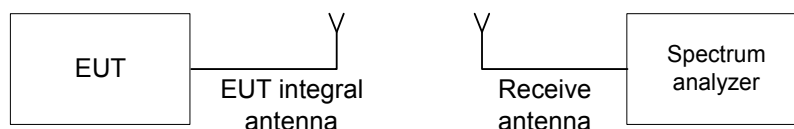
Figure 7.1.1 Setup for transmitter shut down test
