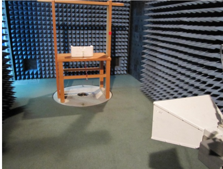
Photograph 8.1.3 Setup for radiated emission measurements
