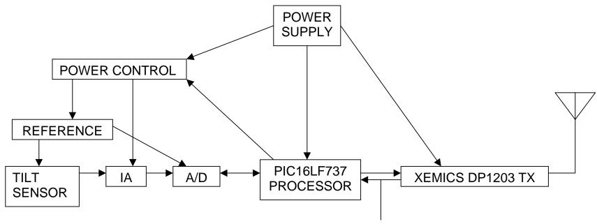
Transmitter contains 39 MHz oscillator, divided down to 1.218 MHz for PIC processor. Transmitter is direct synthesis (zero IF) and production configurable to transmit on 902-928 MHz.
