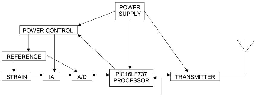
Transmitter contains 39 MHz oscillator, divided down to 1.218 MHz for PIC processor. Transmitter is direct synthesis (zero IF) and production configurable to transmit on 902-928 MHz.
