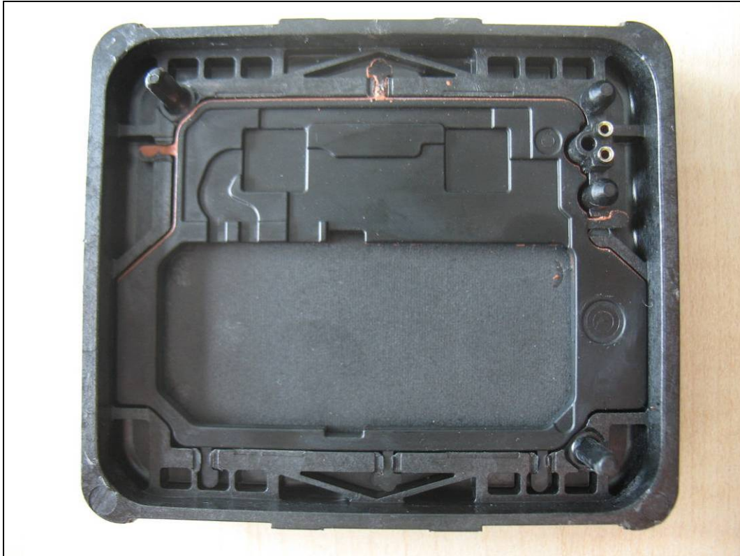
Photo No. 29: cover with absorber material
