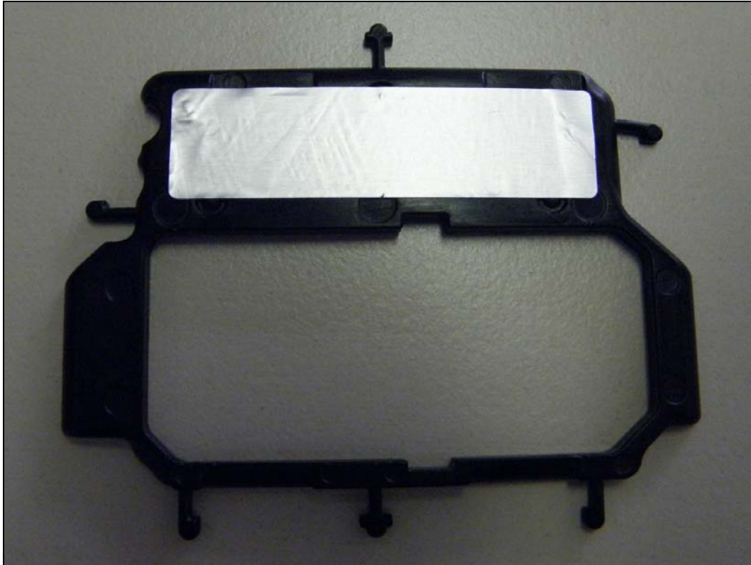
Photo No. 33: alternative absorber with aluminium foil
