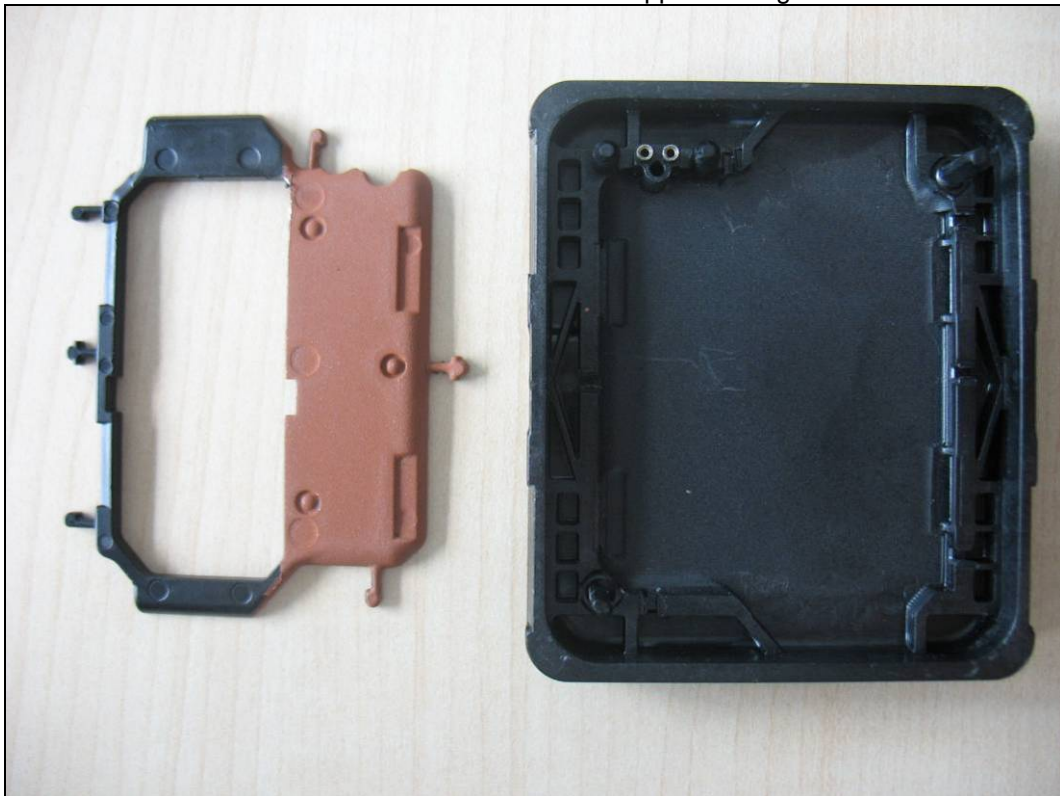
Photo No. 30: absorber with copper coating
