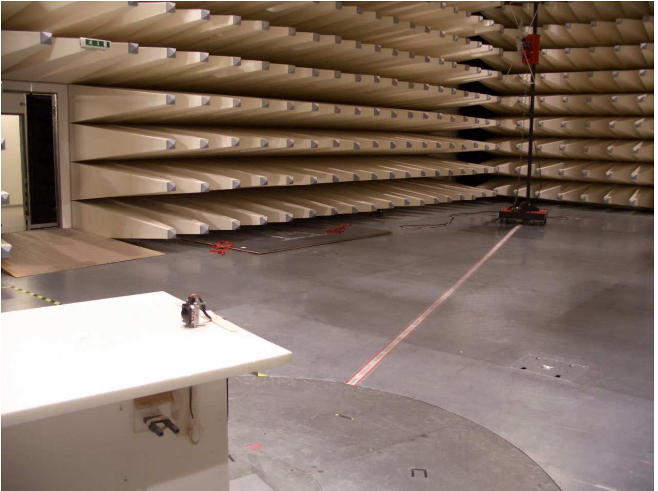
Spurious emission measurement 30 MHz – 1 GHz
