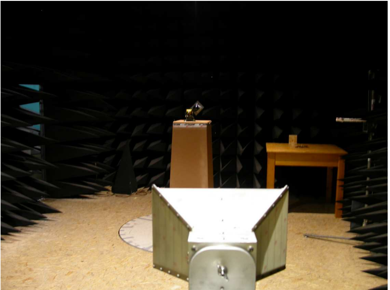
Spurious emission measurement 1 GHz – 12 (18) GHz
