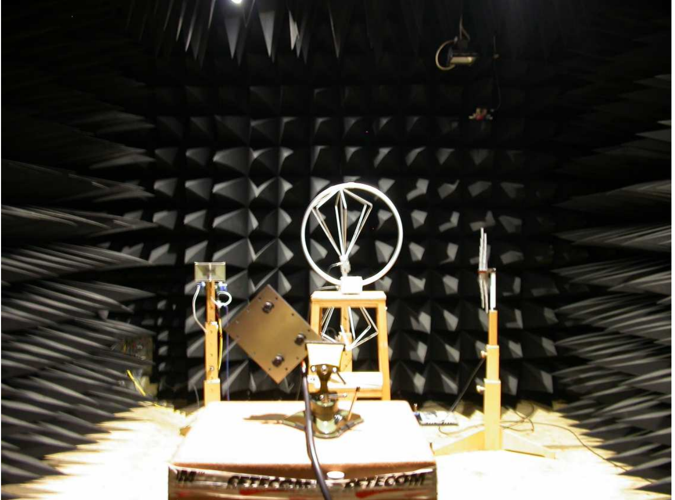
Spurious emission measurement 9 kHz – 30 MHz
