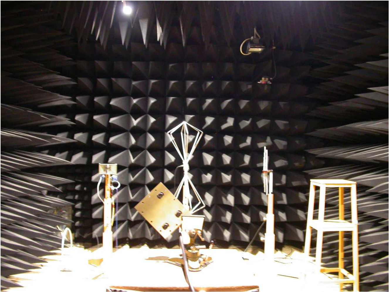
Spurious emission measurement 1 GHz – 12 (18) GHz
