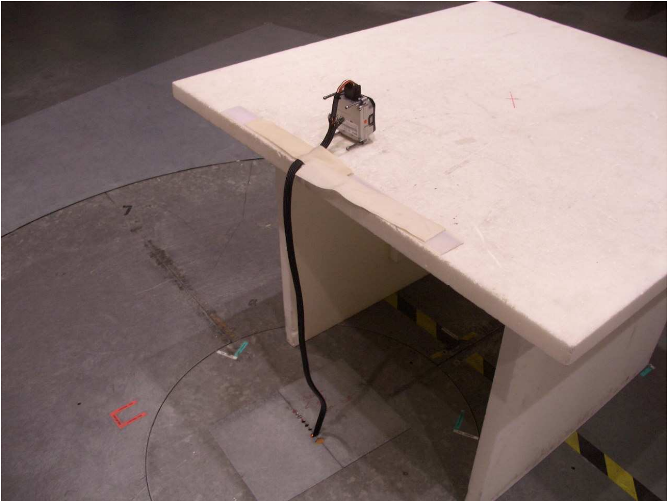
Spurious emission measurement 30 MHz – 1 GHz
