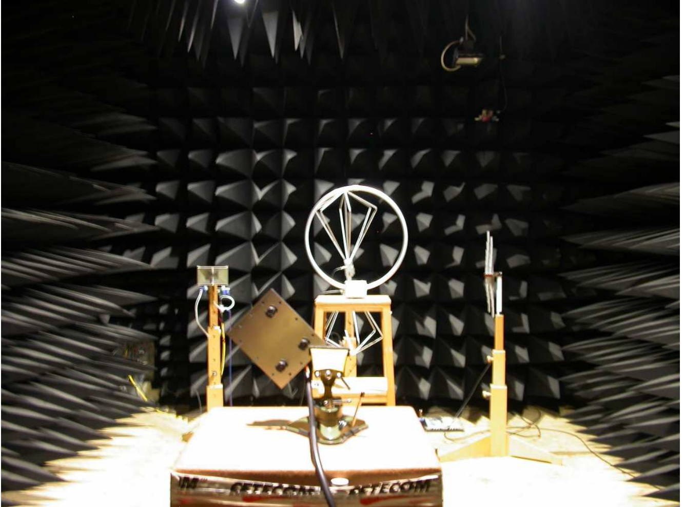
Spurious emission measurement 9 kHz – 30 MHz
