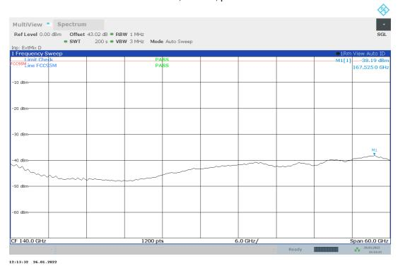
Plot no. 80: radiated emissions 110 GHz – 170 GHz, mode 8, polarization vertical / horizontal
