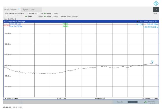
Plot no. 82: radiated emissions 170 GHz – 220 GHz, Mode 7, polarization vertical / horizontal
