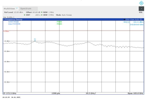
Plot no. 86: radiated emissions 220 GHz – 325 GHz, mode 8, polarization vertical / horizontal
