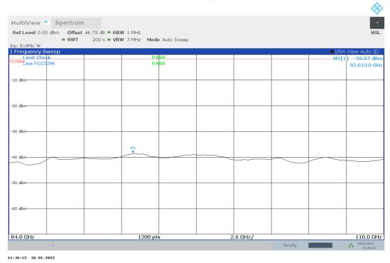
Plot no. 78: radiated emissions 84 GHz - 110 GHz, Mode 9, polarization vertical / horizontal
