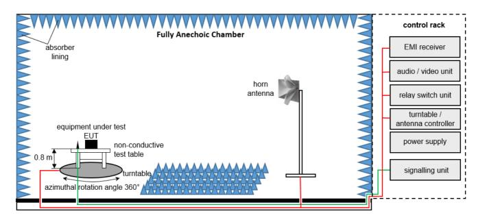
Measurement distance: tri-log antenna and horn antenna 3 meter; loop antenna 3 meter / 1 meter EMC32 software version: 11.00.00
